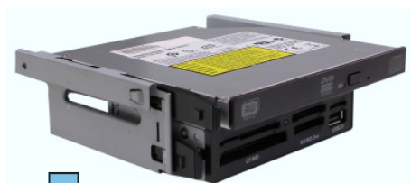
Slide in Rails for drive install
